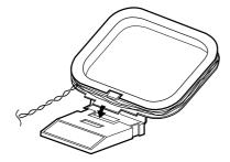
Attach the AM loop to its base by snapping the tabs on the loop into the slot in the base.
